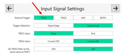
(2) Check appropriate polarity of the external trigger signals.
