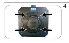
Use the screws removed in 2 to secure the C mount adapter. When fixing with screws, the electronic contacts are springs, so fix while pressing.
