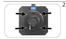
Remove the fixing screws on the lens mount mounted on the ACS.
