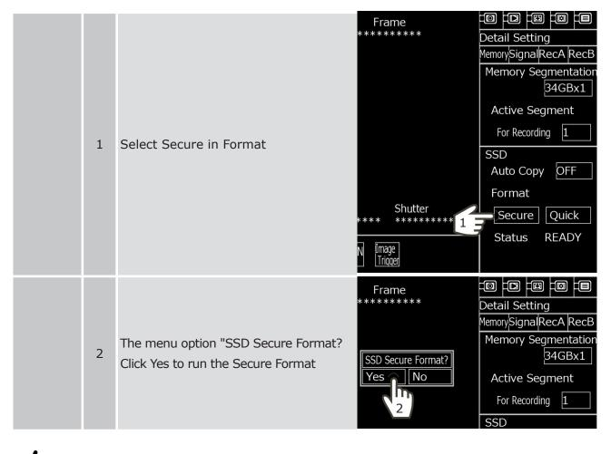
•When the SSD is initialized, the data in the SSD will be erased, so please save the data to external storage or PC if necessary.
