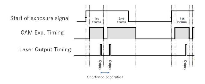
High repetition double pulse laser or Double pulse laser are required for Frame straddling photography with high-speed camera.
