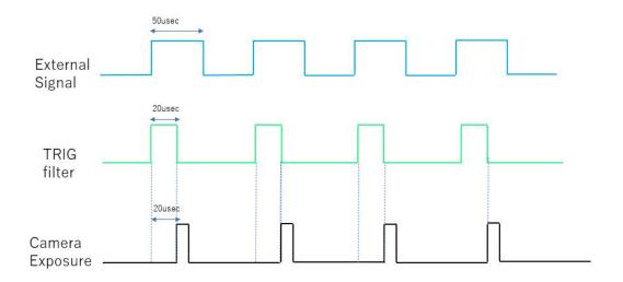
TRIG filter < pulse width of External signal Exposure starts including delay of TRIG filter
