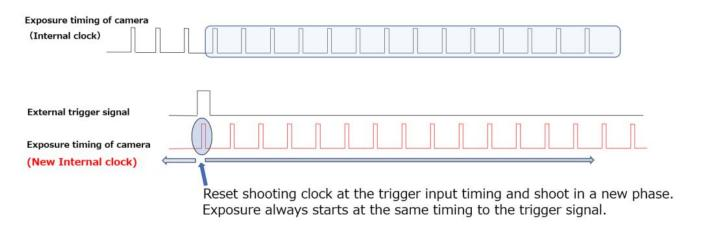
Note: The phase of the shooting clock changes before and after the trigger input. The image before the trigger input is broken.
