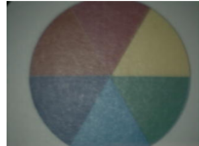
Image captured using a 10mm, right angle (90) line of sight zoom rigid borescope and Xenon lightsource at 5,000 frames per second.
